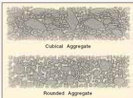
Figure 2: The cubic and round-sides shape of slag aggregates.
