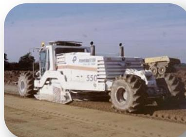
Figure 4: using slag in base and sub-base layer
