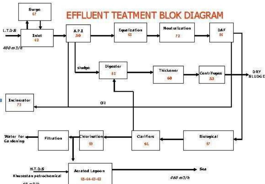
Figure 2: Wastewater treatment process diagram
