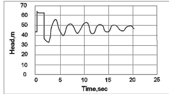
Figure 2: Pressure changes as compared to time according to research conducted by covas et al [10].
