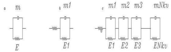
Figure 1: mechanical presentation of a viscoelastic solid substance (a) Kelvin- Voigt (b) three-parameter model of Kelvin- Voigt (c) generalized model of Kelvin- Voigt.
