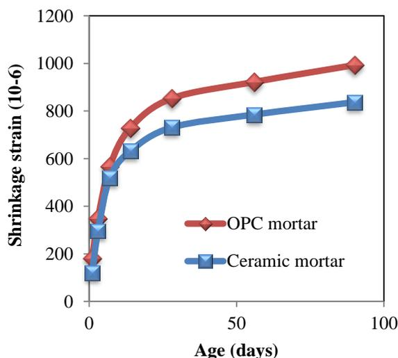
Figure 3: Drying shrinkage of OPC and ceramic mortars
