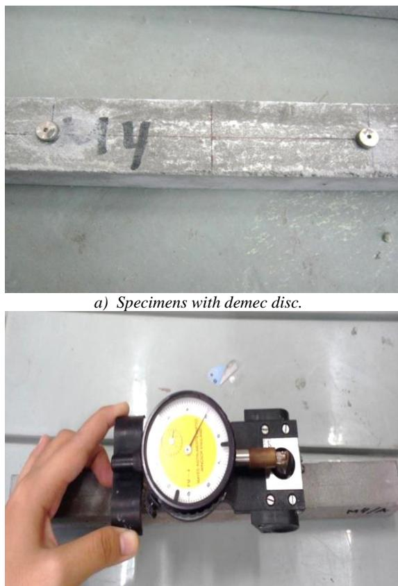
b) Measuring shrinkage using mechanical extensometer.
