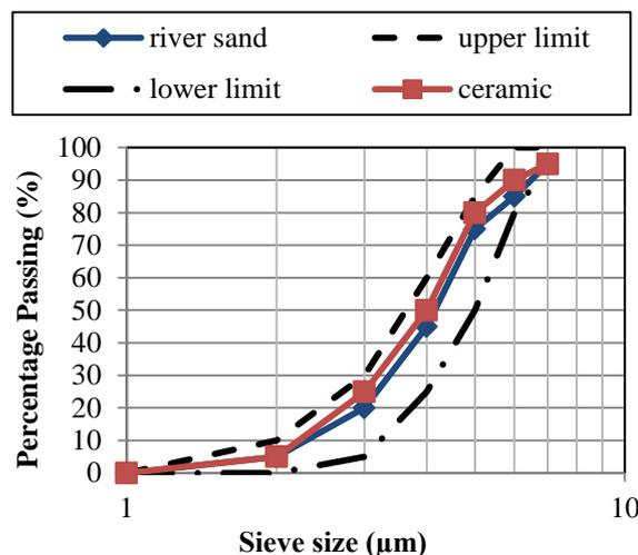
Figure 1: Sieve analysis of fine aggregates according to ASTM C33
