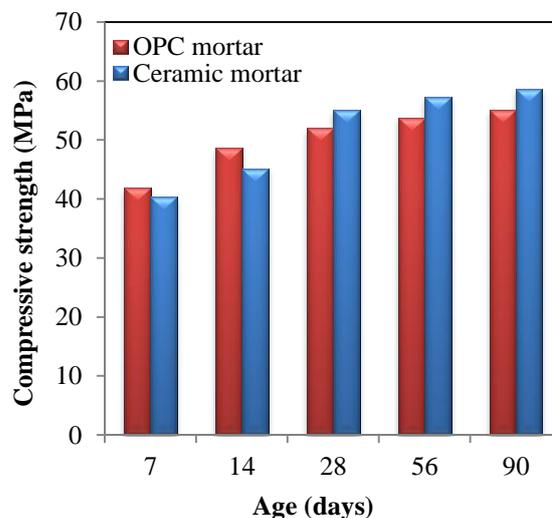
Figure 4: Compressive strength of OPC and ceramic mortars
