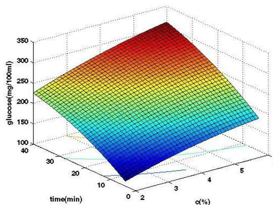
Figure 2. Surface response for glucose concentration in hydrolysis by sulfuric acid as a function of time ad acid concentration
