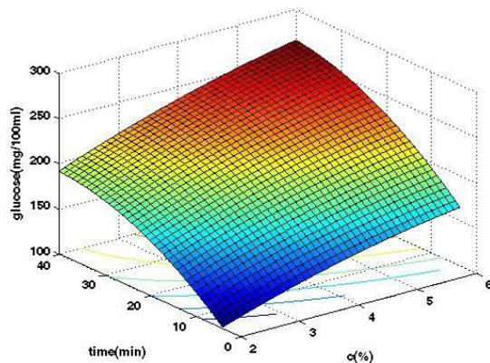
Figure 3. Surface response for glucose concentration in hydrolysis by HCl as a function of time ad acid concentration
