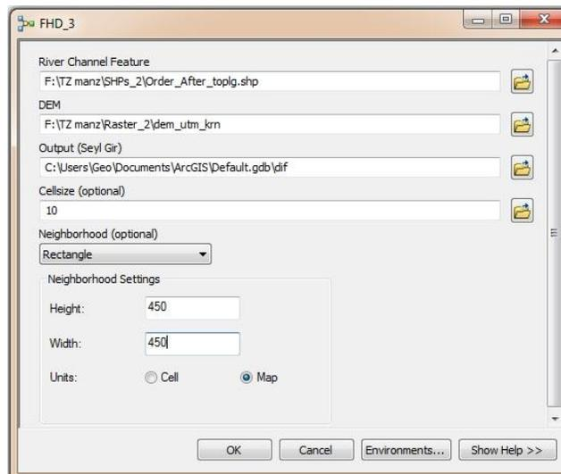
Figure 3: The devised tool to obtain height difference of the channel bed
