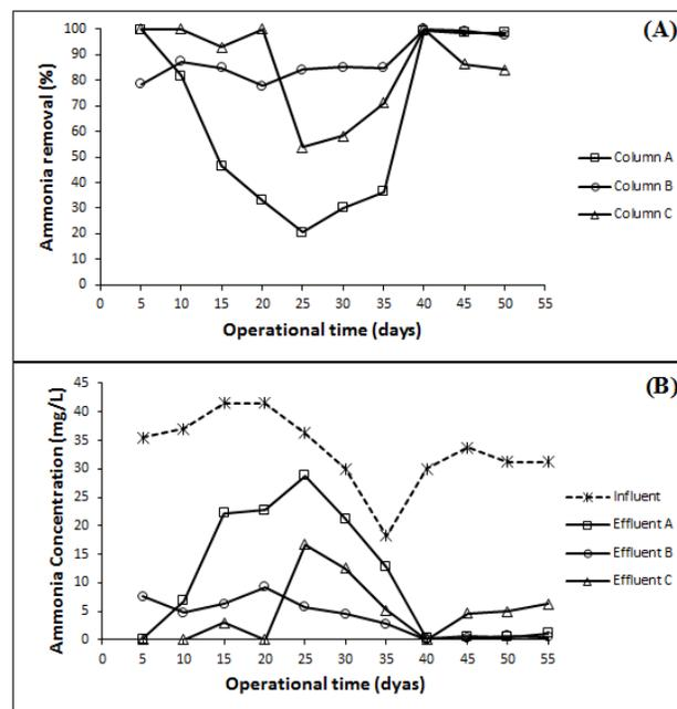
Figure 6: Profile of ammonia removal efficiency (A) and concentration (B) in all columns
