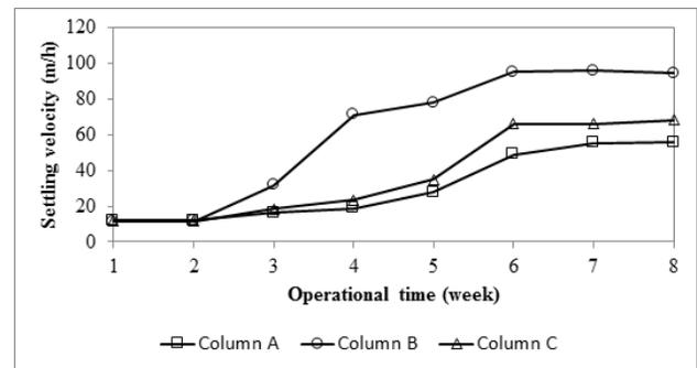
Figure 3: Settling velocity of activated sludge
