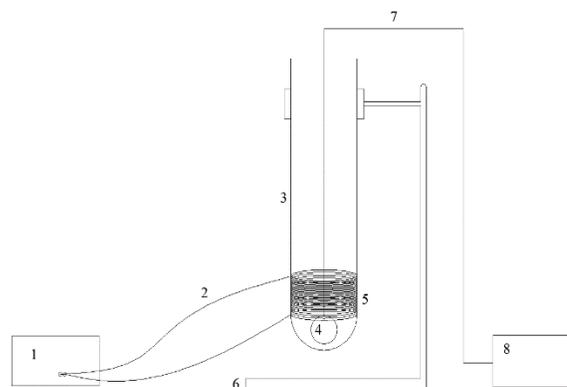
Figure 1: Schematic diagram of the experimental setup (1: DC Power supply, 2: Crocodile clip, 3: Column, 4: Stone diffuser, 5: Copper coil, 6: Retort stand, 7: Tube, 8: Aquarium pump)
