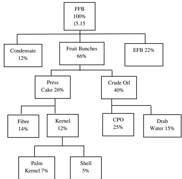
Figure 5: Material balance for 1 t CPO production
