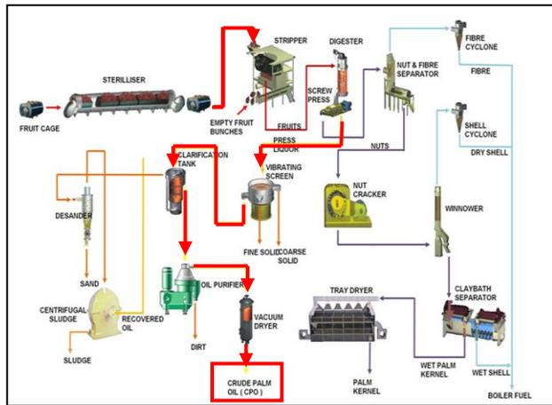
Figure 3: Palm Oil Mill Flow Process Diagram
