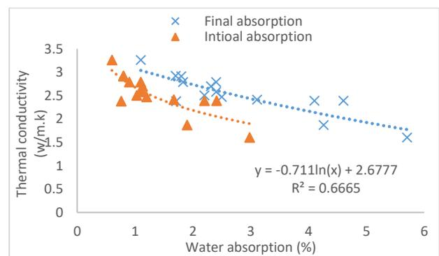
Figure 10: The relation between thermal conductivity and water absorption of normal weight concrete
