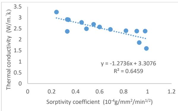
Figure 12: The relation between thermal conductivity and sorptivity of normal weight concrete
