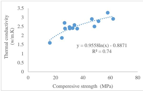
Figure 6: The relation between thermal conductivity and compressive strength of normal weight concrete
