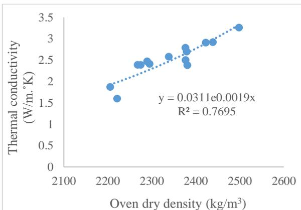
Figure 8: The relation between thermal conductivity and the oven dry density of normal weight concrete
