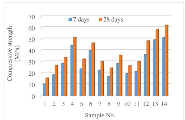
Figure 5: The results from the compressive strength test for 7 and 28 days ages.
