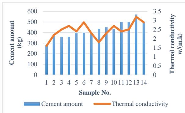
Figure 3: The comparison between thermal conductivity value and cement amount.
