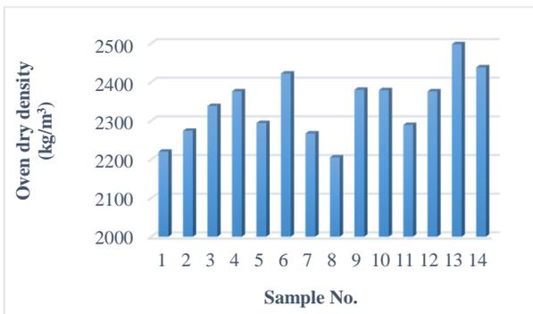
Figure 7: The results from oven dry density test, age 28 days
