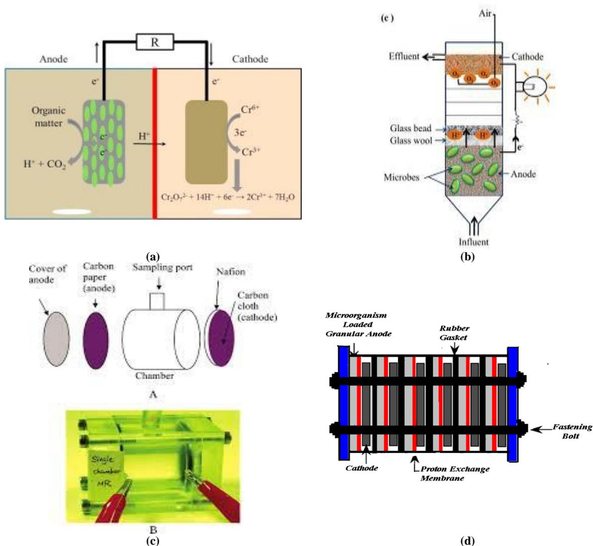
Figure 1: Schematic diagram of (a) Dual chamber MFC (b) Up-flow MFC (c) Single chambered Air-cathode MFC (d) Stacked MFC
