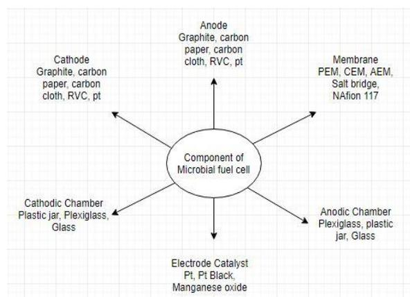
Figure 2: Components of microbial fuel cell
