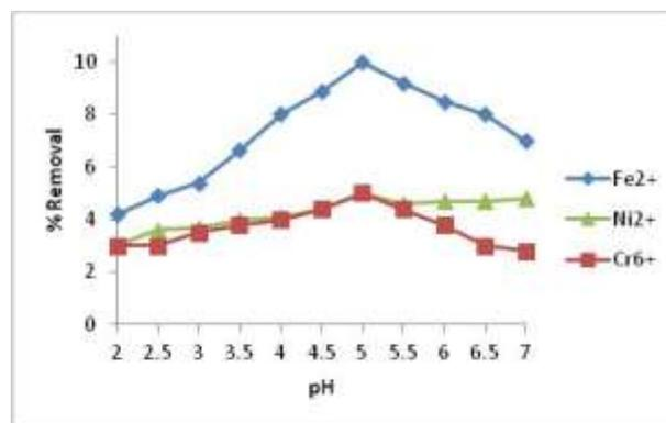
Figure 1: Effect of pH on removal percentage of metal ions
