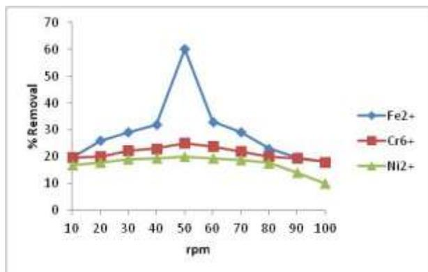
Figure 3: Effect of rotor's rotation on removal percentage of metal ions
