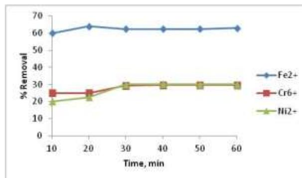
Figure 4: Effect of contact time on removal percentage of metal ions
