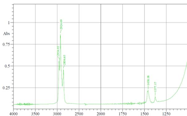
Figure 1: FTIR-Spectra of petrodiesel sample
